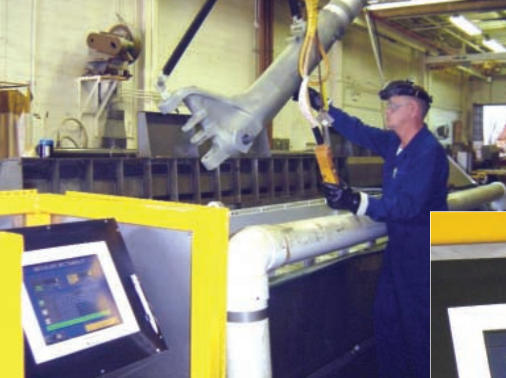
LEFT: Tom Adams shown anodizing an EA-6B main landing gear in modified anodizing tank.
