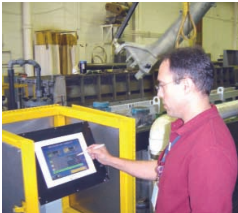
At the Surface Finishing Shop, Ruben Prado enters a “strategy” into the Metalast™ Integrated Process Controller prior to anodizing an EA-6B main landing gear.
